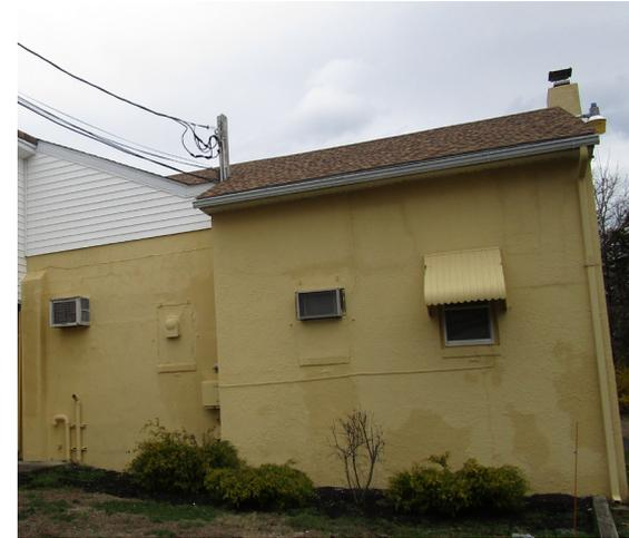
A rain garden can be installed in the turfgrass area on the south side of the building to capture, treat, and infiltrate stormwater runoff from the roof. A preliminary soil assessment suggests that the soils have suitable drainage characteristics for green infrastructure.
